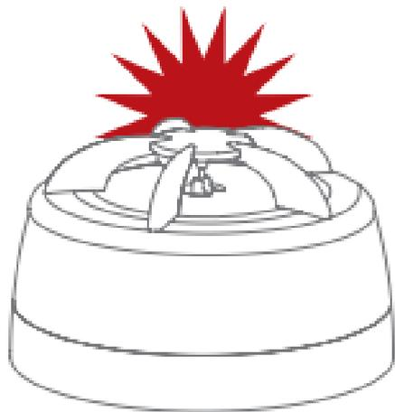
Please note that when the alarms are placed in 'Learn Mode' they can't be inserted into the mounting base.
