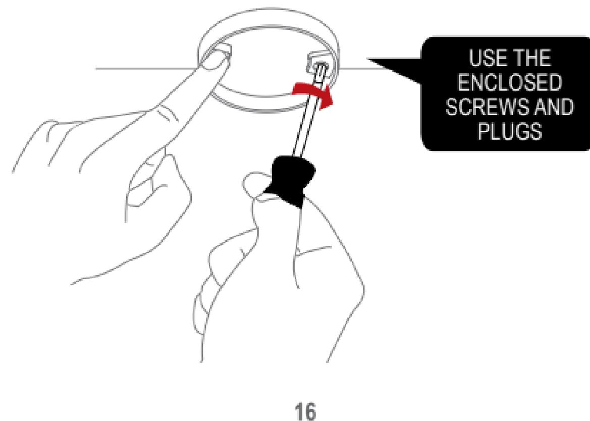
Once the mounting base is installed, attach the alarm by twisting clockwise until it clicks. If the battery is either missing or inserted incorrectly, or the switch is in 'Learn Mode', the heat alarm will not be able to click into the mounting base.
